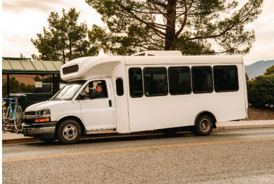
Figure 18: Cutaway bus. Image: National Rural Transit Assistance Program
