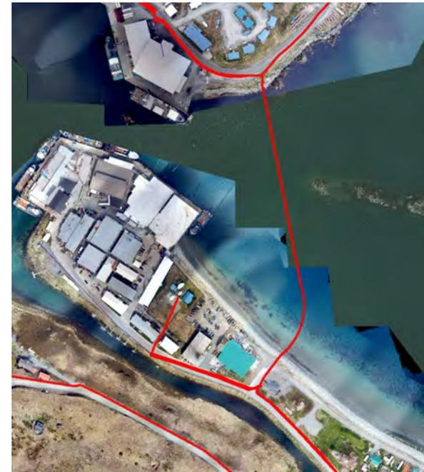
**Project Description:** The Electric Utility relies on the 34.5 kV sub-transmission system to deliver power to major Industrial loads and to the Town Substation. It uses two existing feeders: one crosses Iliuliuk Bay between East Point Road and Bay View Avenue and is near the end of its lifespan. Replacement is required.
